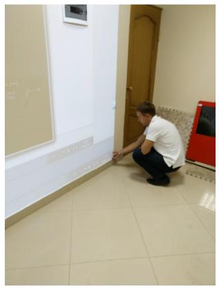
Pic. 24 Calibrating the bottom right corner (wall)
