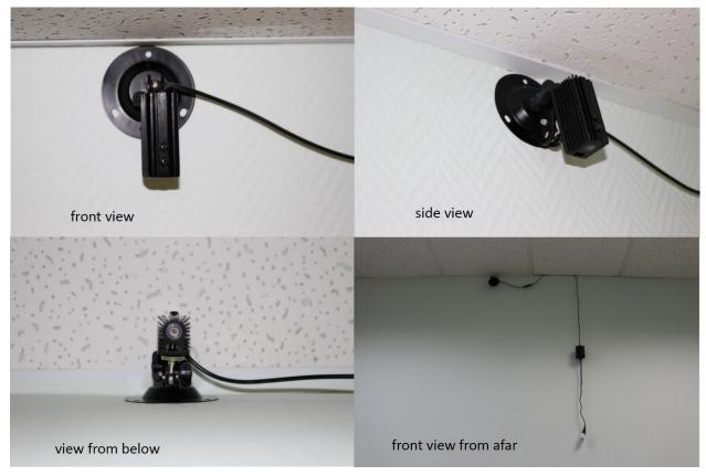
Pic. 5 (Option 1) Mounting the infrared sensor on the wall
