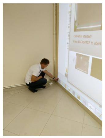
Pic. 22 Calibrating the bottom left corner (wall)
